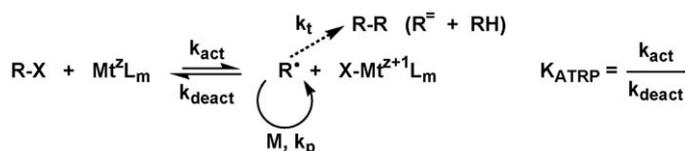
Scheme 1. Atom transfer radical polymerization.
