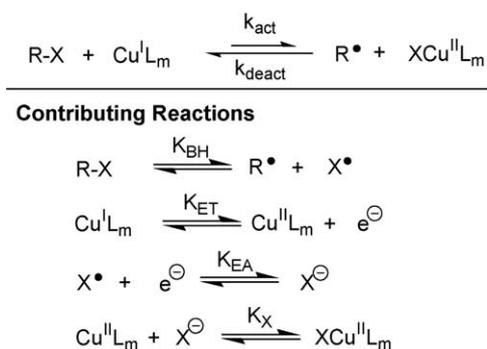
Fig. 1. Representation of atom transfer as a combination of a C–X bond homolysis of alkyl halide (RX), two redox processes, and a heterolytic cleavage of Cu<sup>II</sup>–X bond. L represents a ligand (adapted from Ref. [71]).
