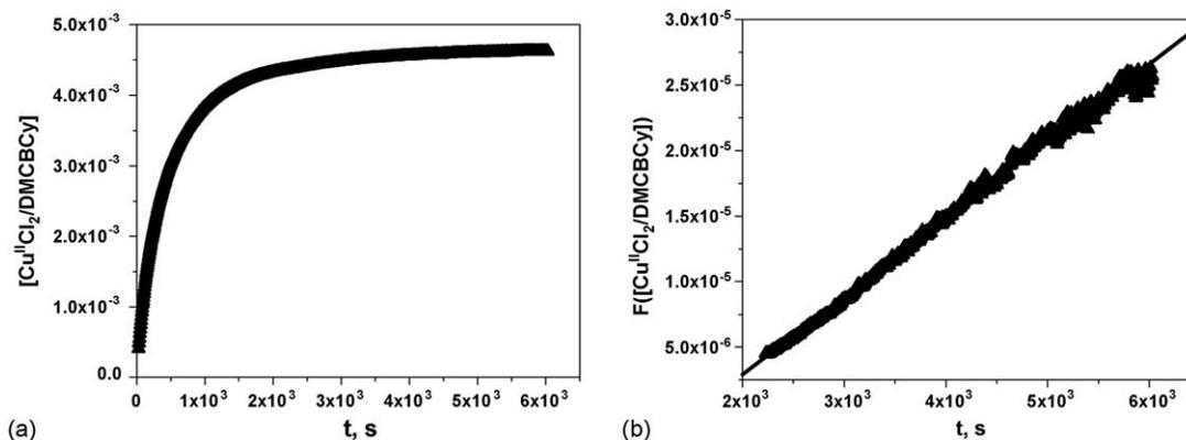
Fig. 3. Determination of  $K_{\text{ATRP}}$  for the reaction of  $\text{Cu}^{\text{I}}\text{Cl}_2/\text{DMCBCy}$  (5 mM) with  $\text{MClAc}$  (5 mM) in  $\text{MeCN}$ : (a) accumulation of deactivator with time; (b) plot of  $F([\text{Cu}^{\text{II}}\text{Cl}_2/\text{DMCBCy}])$  against time (equilibrium reached in ca. 2000 s).
