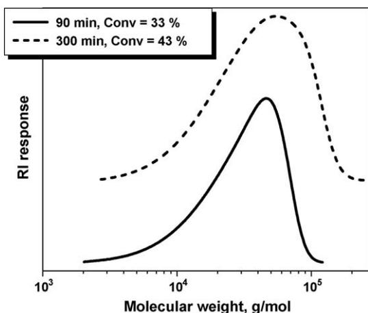
Fig. 4. SEC traces of poly(*n*BA) produced in the solution ATRP of *n*BA using [*n*BA]:[MBP]:[Cu<sup>I</sup>Br/DMCBCy] = 500:1:1 at 75 °C. The amount of butanone was 33 vol.%.
