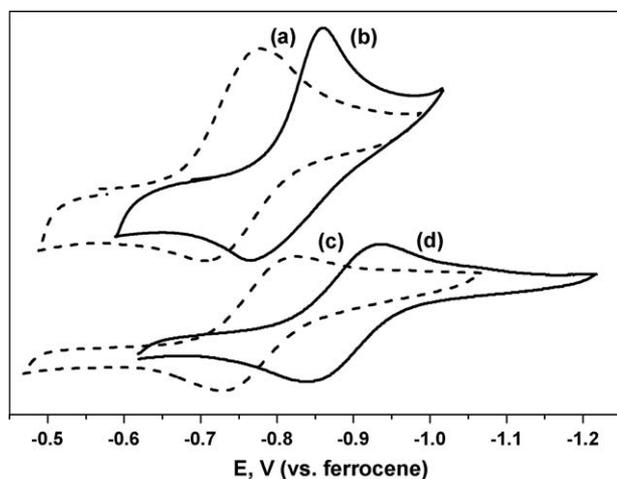
Fig. 2. Cyclic voltammetry of Cu<sup>II</sup>X<sub>2</sub>/Me<sub>6</sub>TREN (X=(a) Br and (b) Cl) and Cu<sup>II</sup>X<sub>2</sub>/DMCBCy (X=(c) Br and (d) Cl) in acetonitrile; 0.1 M Bu<sub>4</sub>NPF<sub>6</sub>, 1.0 mM Cu<sup>II</sup>X<sub>2</sub>/L; scan rate = 0.10 V s<sup>-1</sup>.
