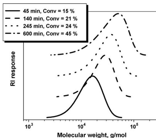
Fig. 5. SEC traces of poly(*n*BA) produced in the bulk ATRP of *n*BA using [*n*BA]:[MBP]:[Cu<sup>I</sup>Br/DMCBCy] = 500:1:1 at 30 °C.
